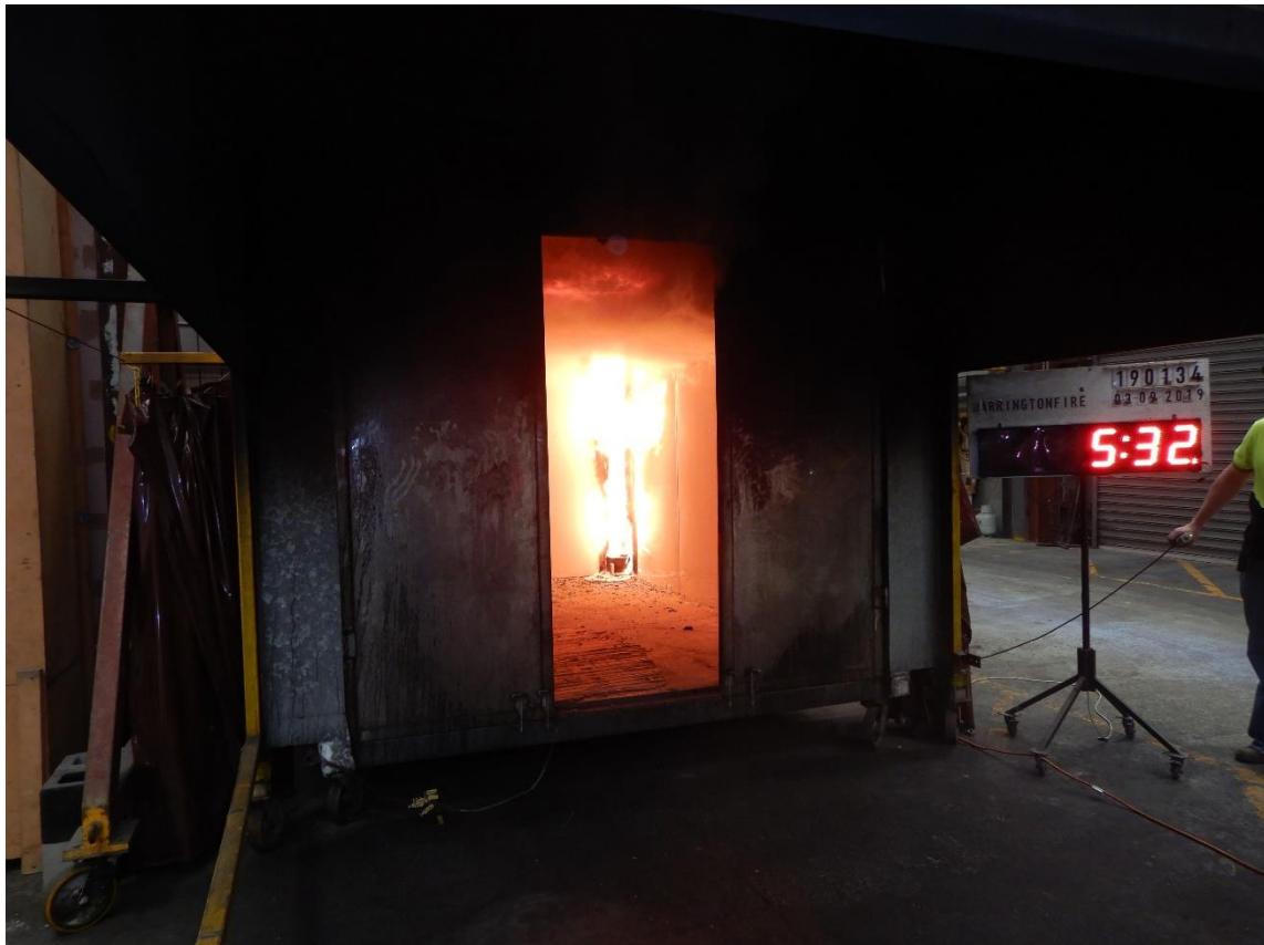
Figure 26 The specimen 05 minutes 32 seconds after burner ignition with a burner output of 100 kW
