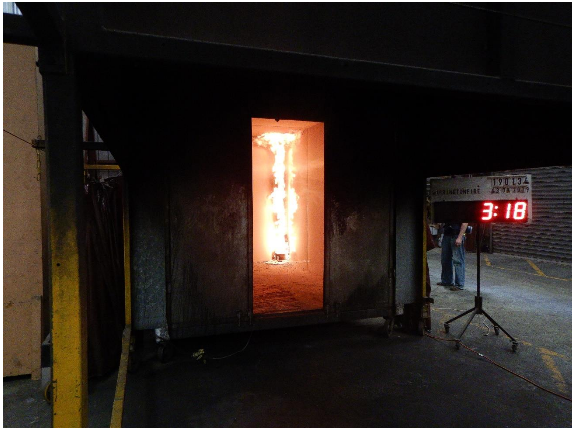
Figure 24 The specimen 03 minutes 18 seconds after burner ignition with a burner output of 100 kW
