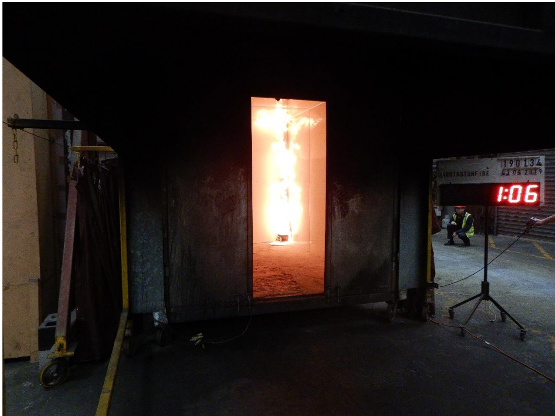
Figure 22 The specimen 01 minute 06 seconds after burner ignition with a burner output of 100 kW
