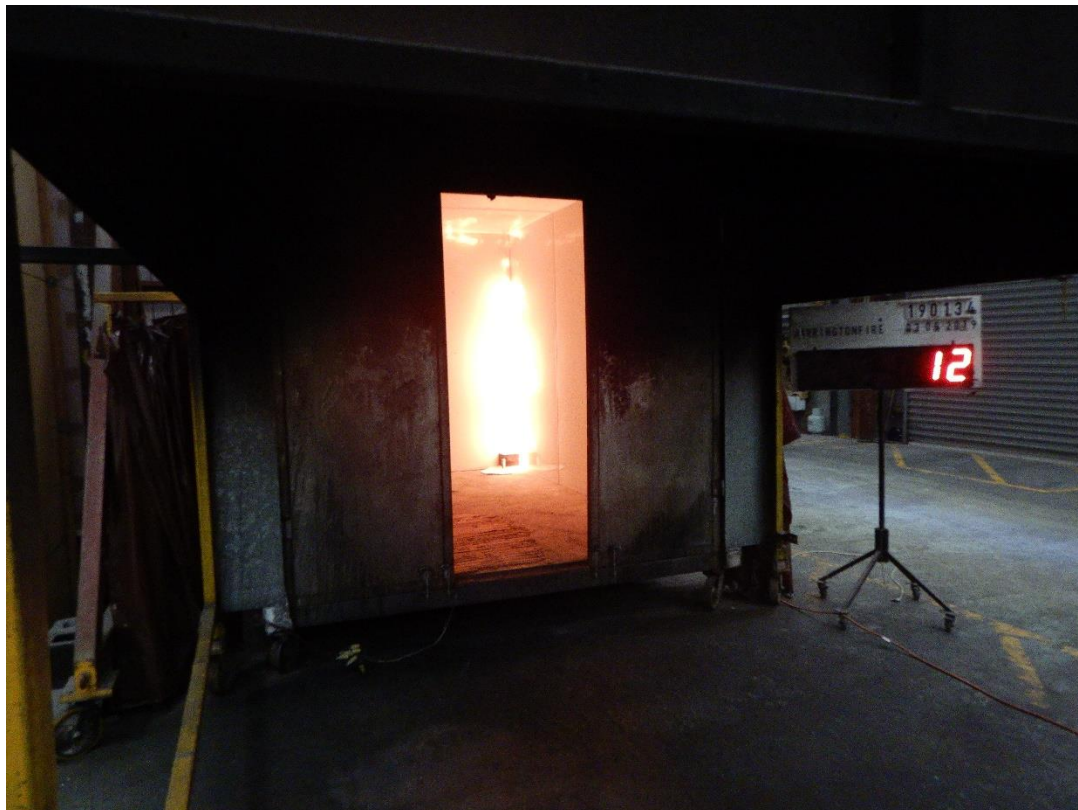
Figure 20 The specimen 12 seconds after burner ignition with a burner output of 100 kW
