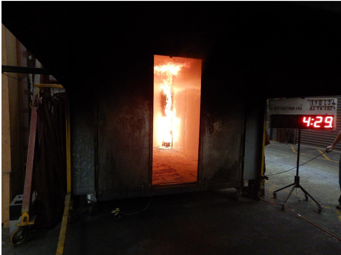
Figure 25 The specimen 04 minutes 29 seconds after burner ignition with a burner output of 100 kW
