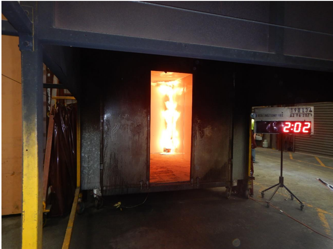
Figure 23 The specimen 02 minutes 02 seconds after burner ignition with a burner output of 100 kW
