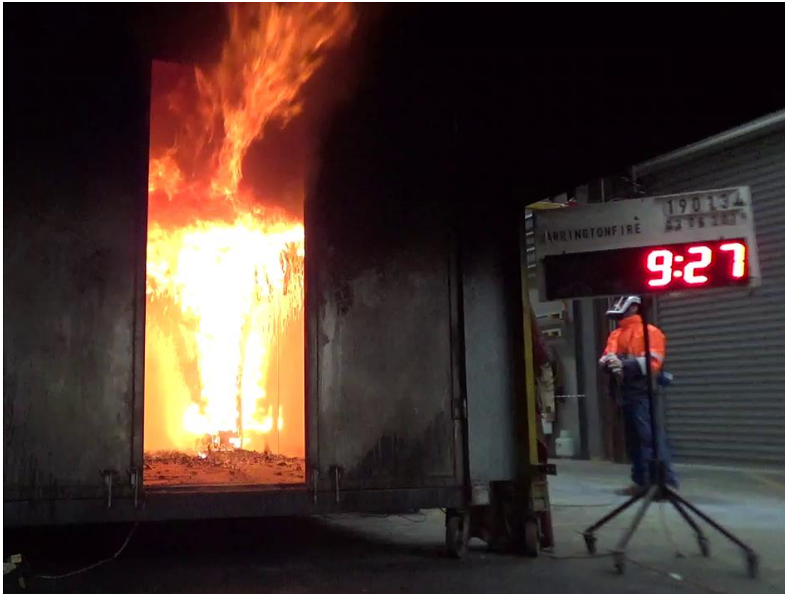
Figure 29 The specimen 09 minutes 27 seconds after burner ignition with a burner output of 100 kW
