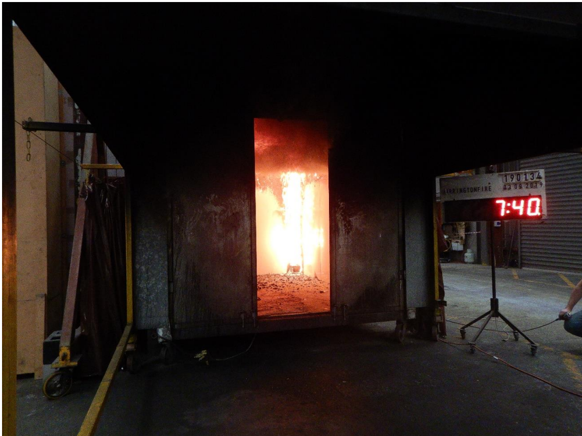
Figure 28 The specimen 07 minutes 40 seconds after burner ignition with a burner output of 100 kW
