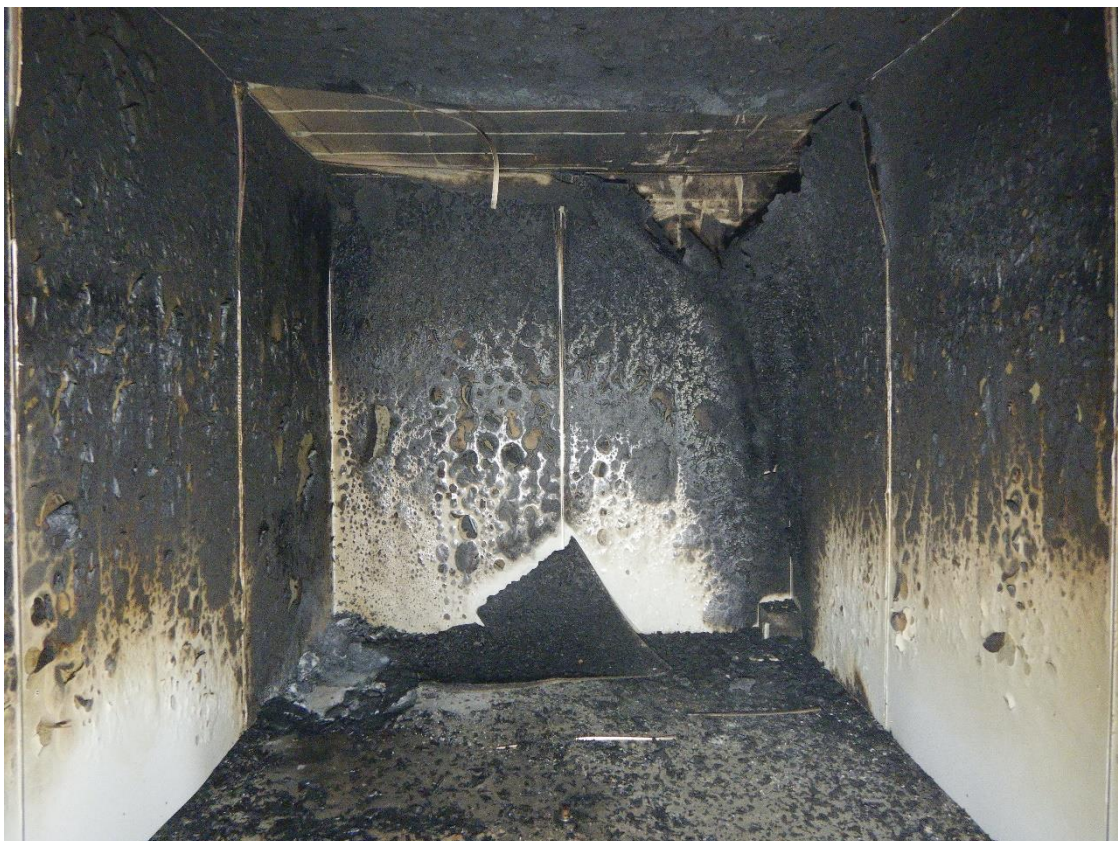
Figure 30 The specimen after the reaction-to-fire test
