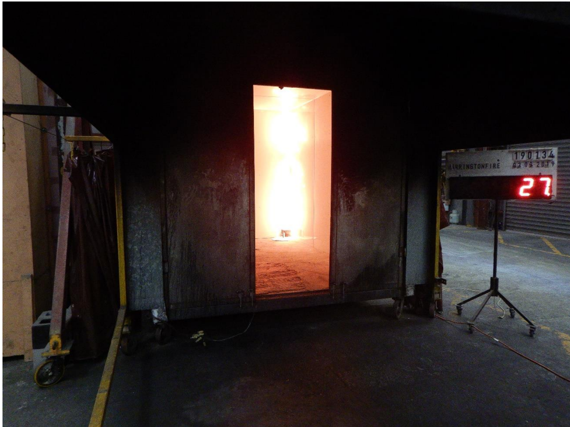
Figure 21 The specimen 27 seconds after burner ignition with a burner output of 100 kW
